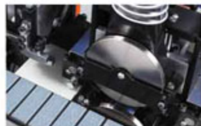
Guillotine Shears Coiled material up to 3 mm in thickness can be trimmed by the guillotine shears.
