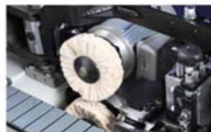
Buffing Unit The buffing unit leaves a super finish on ABS and PVC edging, and removes any discoloration on the edges, which is especially noticeable when working with dark edge material.
