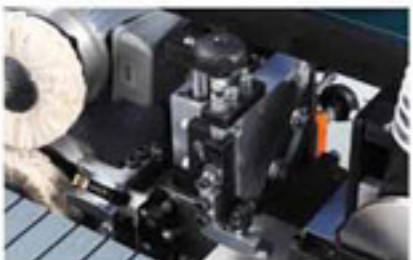
Scraping Unit - Radius Scraping Unit The scraping unit fine-tunes the edge radius and removes excess glue.
