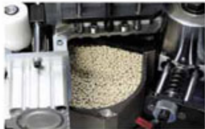
Glue Pot The 1.2 kg Teflon-coated glue pot is designed for EVA hot-melt glue. The glue is applied with an adjustable glue roller.
