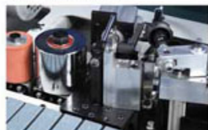
Guillotine Shears Coiled material up to 3 mm in thickness can be trimmed by the guillotine shears.
