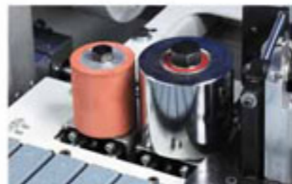
Pressure Roller The pressure roller unit is to improve the bond between the edge and the material. The unit is mechanically spring-loaded and due to the "Quick" setup system, can be adjusted exactly to the required edge thickness.
